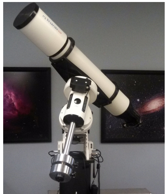
The mount below the 3600 in capacity is the AP 1600. This gem (he he he!) sports a 220 lb. capacity and is not so portable at 114 lbs. It is shown with a nice 175mm Apochromatic refractor (well – nice and huge!).
