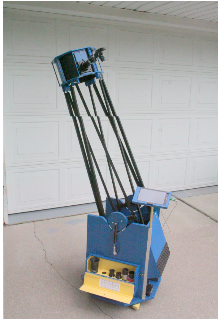
Above: Completed telescope. Note the eyepiece box and the stalk for Don's tablet.
